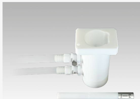
| TEMPERED MEASURING CELL (0°C to 90°C)
