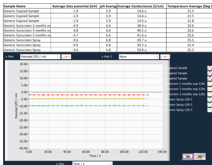
Figure 3: Comparative Analysis of Zeta Potential in Expired About-to-Expire, and Long-Shelf-Life Sunscreen Spray
