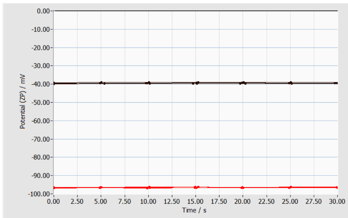
Figure 3 shows zeta potential in millivolts, collected over a 30 second time period. The black lines represent undiluted ink, where the red lines represent the same ink at 1 : 10,000 dilution.
